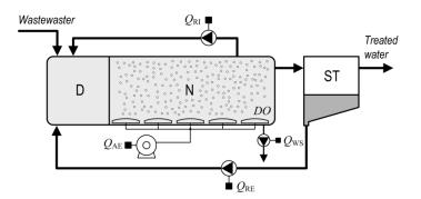
The **art-ICA** controllers have been developed for application to pre-denitrification / nitrification plant designs (also known as conventional BNR systems), which represents the most common type of plant-layout found in full-scale BNR WWTPs in Spain, Portugal and the European Union.
